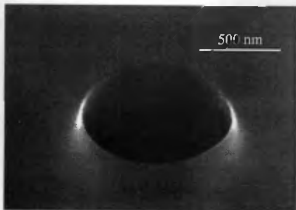
Figure 4.4: 1 \mu\text{m} lens bore fabricated in a silicon membrane with very vertical side walls and a roughness of less than 10 nm.
