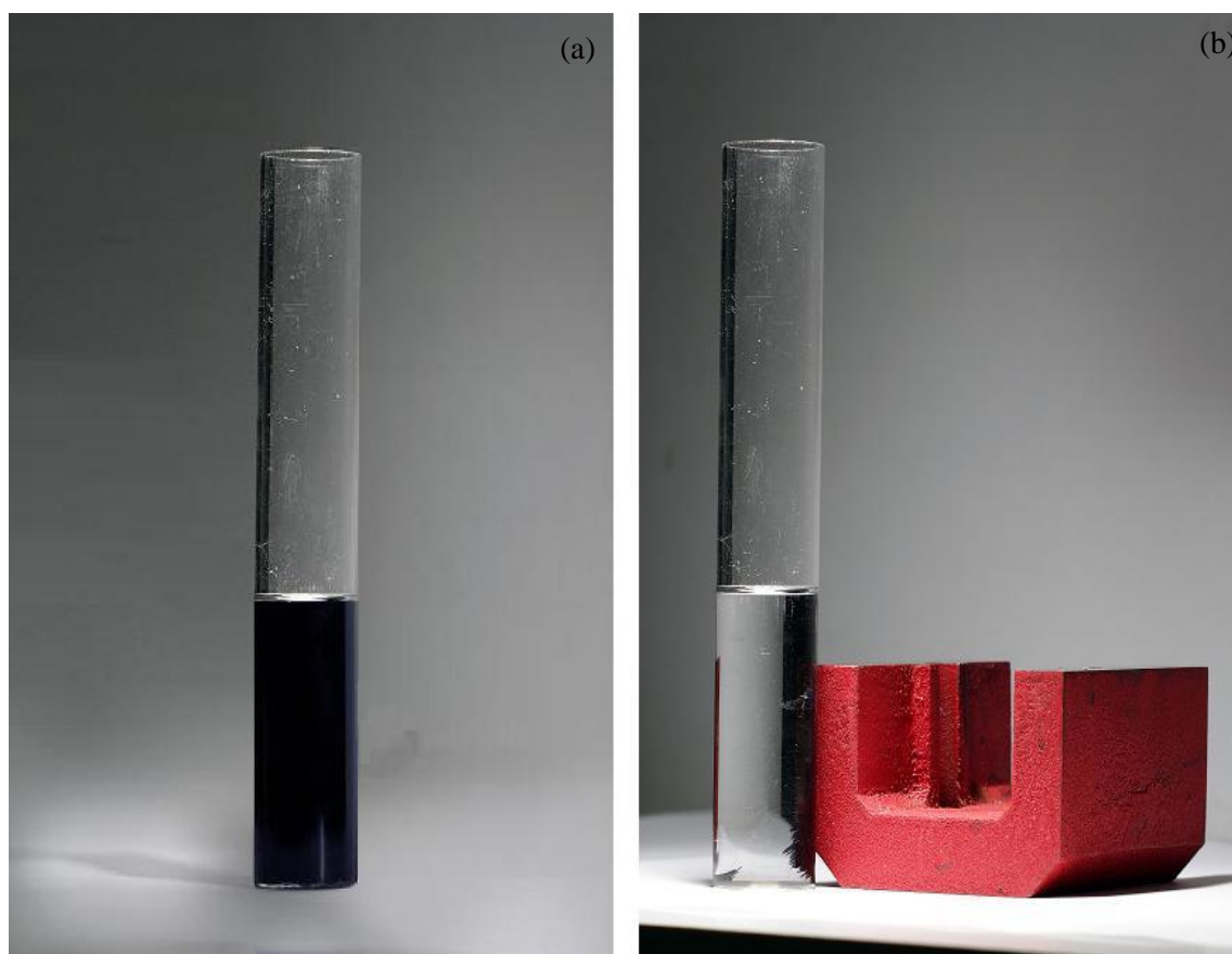
Figure 42. Superparamagnetic core-shell-type \text{Fe}_3\text{O}_4/\text{Ru} nanoparticles dispersed in n-BuOH (a) and placed on the glass wall by an external magnet (b)
