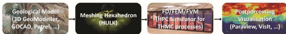
Figure 46: Ideal workflow for 3D numerical modelling based on AMR algorithm, C++ libraries and MPI architecture CPU/GPU.
