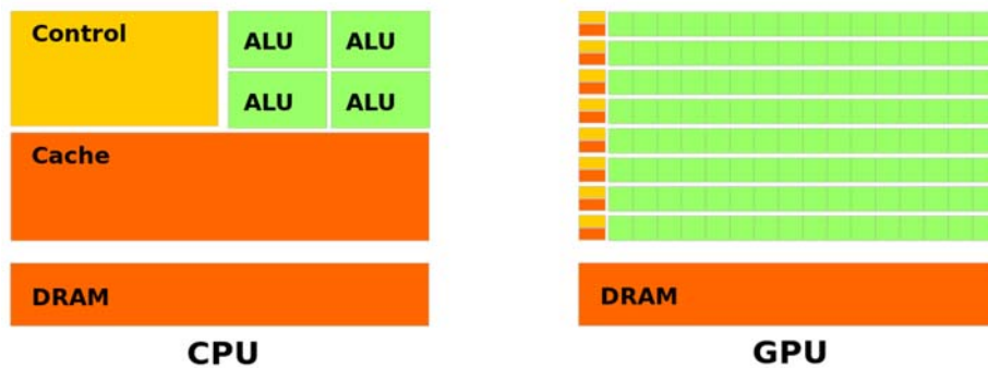
Figure 8: CPU architecture is designed for serial computations. For this reason it dedicates more chip space to flow control and memory operations. Multi-GPU architecture gives priority to arithmetic intensive operations. Much more Arithmetic Logic Units (ALUs) are built in GPU chips. Cache memory for memory operations and flow control units are limited causing GPUs to be inefficient in comparison to CPUs for serial processes (NVIDIA, 2017).
