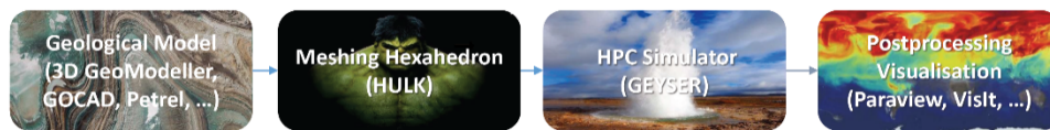
Figure 33: Our workflow for 3D numerical modelling based on “High Performance Computing” algorithms using CPU, GPU or MIC clusters.
