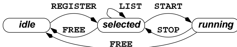
Figure 3.4 – State machine of a SPLAY job on a host.
