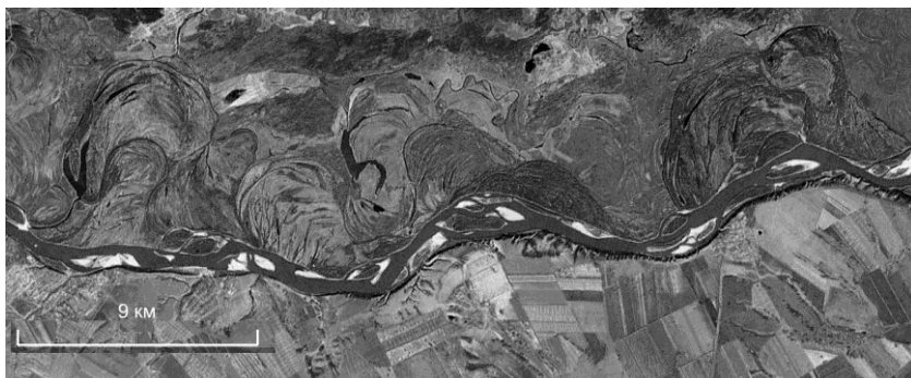
Figure 16. Channel transformation of the Upper Ob' River (No. 53 in Table 3) from steeply meandering with small meanders into gently meandering with large meanders and point bars. A segment with one-sided floodplain.
