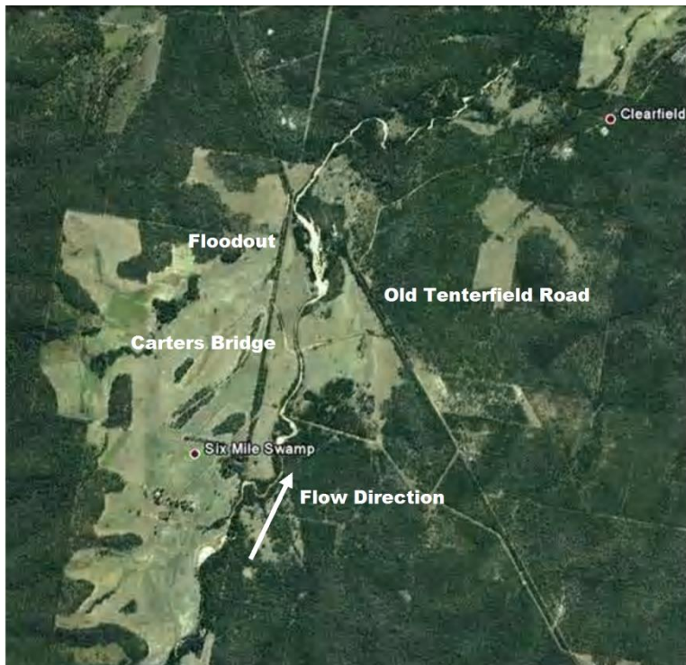
Figure 8. The floodout in August 2006 has contracted and revegetated since 1955 (compare with Figure 7). Also note that sand extends a long way downstream of the floodout.
