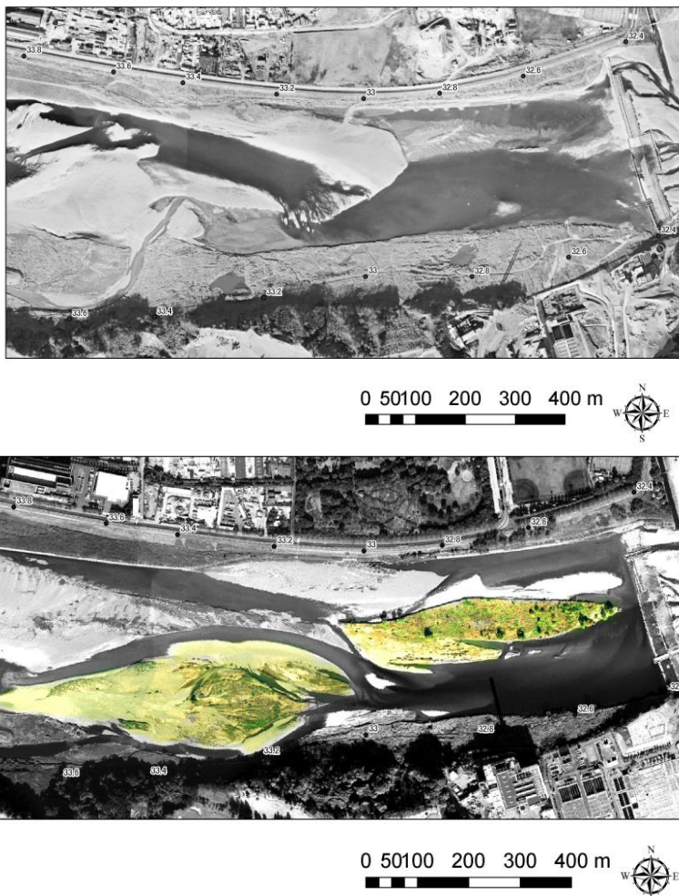
Figure 5. Temporal variation of vegetation in Tama River floodplain, Tokyo. The top photo was taken in 1974, whereas the bottom photo was taken in 2001 in the same bar.
