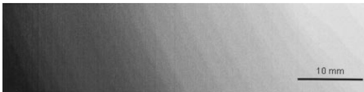
Fig. 2. Range image of Anadonta cygnea (L.) surface. Four cm 2 surface (4 × 1 cm) of shell has been digitized using 3D scanner (REPLICA 500). This surface covers at least two winter crests.
