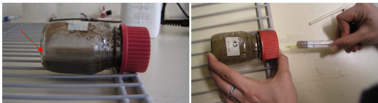
Figure IV. 6. Red arrow in the left picture shown the liquid phase which is going to be sampled as in picture right.
