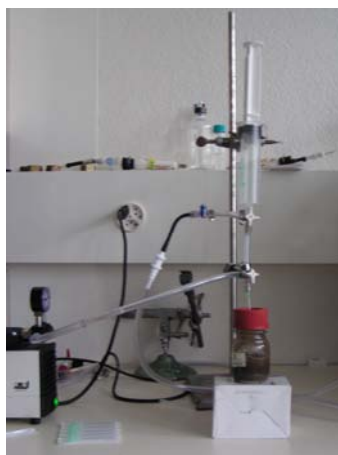
Figure IV. 4. Bottles preparation for 15 N-isotopes incubations containing A) homogenized soil fraction and anoxic sterile water; B) Gas removal by vacuum and nitrogen gas input (gas flow connected with the top of the bottle by a syringe).
