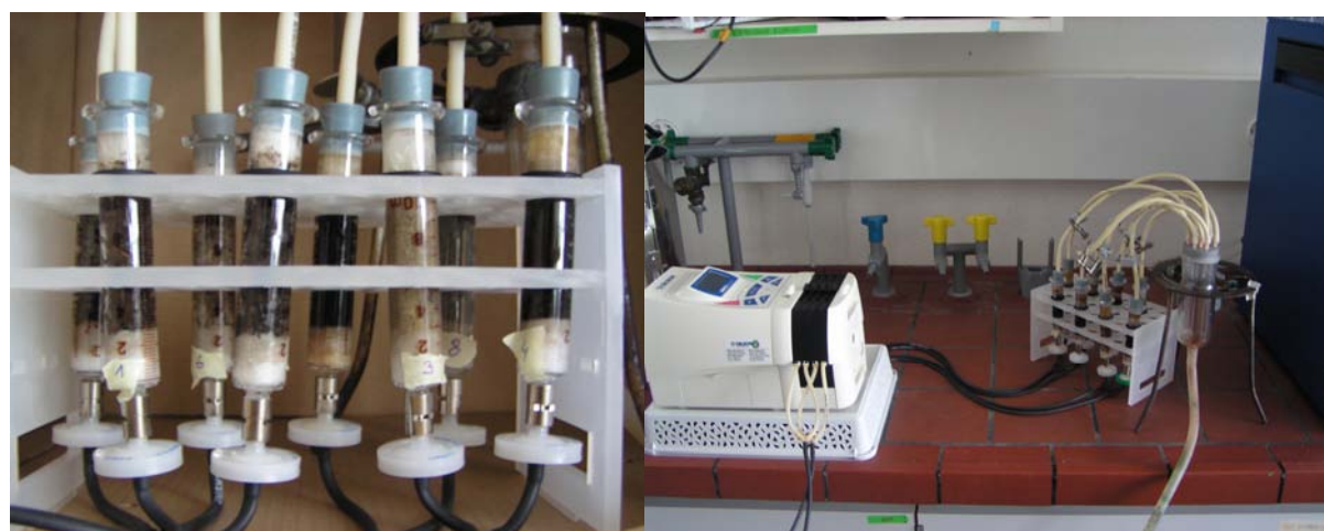
Figure VI. 2. The eight microcosm enrichment cultures (left) with the pump delivering continuously the anoxic mineral medium (right).
