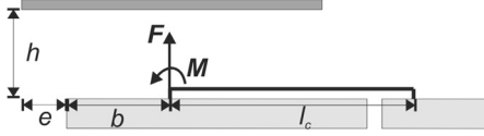
Fig. 3. Suspension model. The electrostatic forces acting on the mirror are replaced by a resulting force and moment acting on the endpoint of the suspension cantilever.
