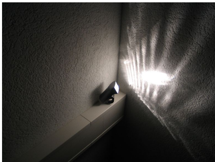
Figure 4.16: Multipath in standard photography. A flashlight is positioned near a corner. Although the flashlight illuminates only the right wall, the left wall is also visible. Most of the light incident on the right wall is diffused. Some of this light illuminates the left wall, and a fraction of this light is diffused towards the camera.
