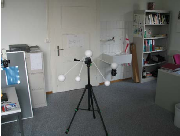
(a) Calibration object (illustrative color image). 5 highly reflective balls, assembled into a three-dimensional object. Ball centers are used as reference points.
