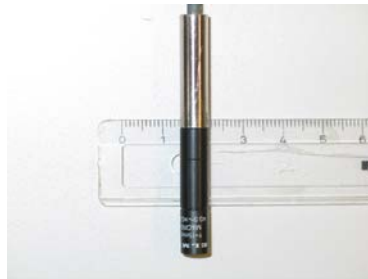
Figure 3.4: Kappa CH-166 camera head with 15mm objective.
