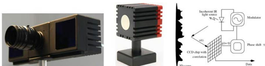
Figure 2.16: Left: PMDTec/ifm electronics CamCube sensor; Middle: MESA SR4000 sensor; Right: The ToF phase-measurement principle. - Excerpt from Kolb et al. [69].
