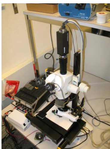
Figure 3.3: Depth from focus 3D microscope: Leica MZ-12 with Pulnix TM-1001 camera.
