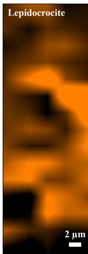
Supplementary figure 8: Chemical maps of goethite (green) and lepidocrocite (orange), obtained by Raman spectroscopy on the untreated samples presenting a natural urban corrosion.
