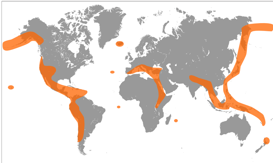
Figure 1.2: The world's main hot temperature zones where geothermal power can be harnessed from hydrothermal reservoirs. The zones are located along active plate boundaries or hot spots. Large parts coincide with the Ring of Fire in the basin of the Pacific ocean that is associated with numerous earthquakes and volcanic arcs. Based on information from the Icelandic National Energy Authority.
