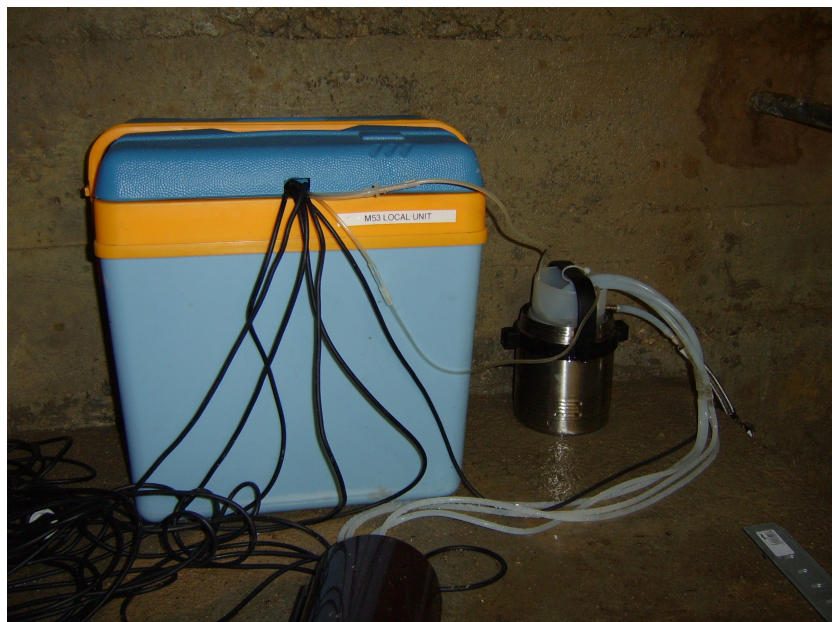
Fig. 13: Radon and CO 2 sensors enclosed together with the pump and electronics in a watertight box.
