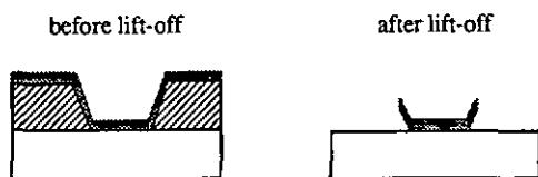
Fig. 5.5: Schematic illustration of microcrack at the top of the metal layer.
