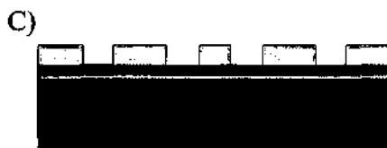
Fig. 3.12: Development of the resist layer
