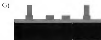
Fig. 3.30: Stripping of the resist mould.
