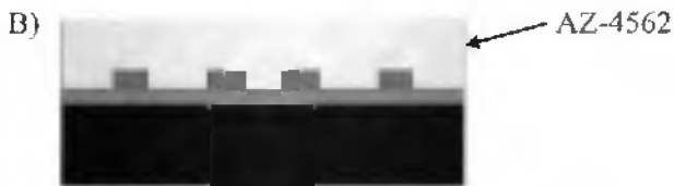
Fig. 3.26: Positive resist layer directly spun on the electrodeposited nickel wheel.
