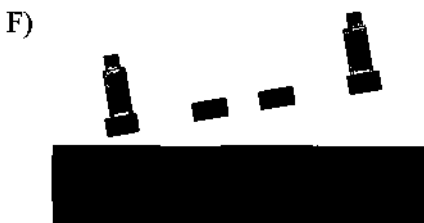
Fig. 3.21: Structures released by sacrificial etch of the Ti layer in HF.
