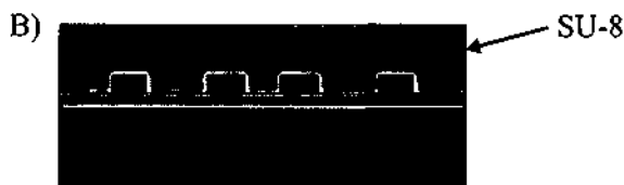
Fig. 3.17: SU-8 layer directly spun on the electrodeposited nickel wheel.
