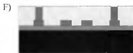
Fig. 3.29: Electroplating of the nickel in the resist mould.
