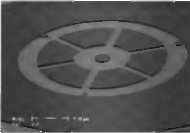
Fig. 3.13: A 38 \mu\text{m} thick photoresist mould of the wheel, before the nickel electrodeposition.
