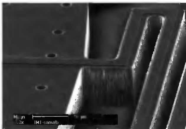
Fig. 2.16: Detailed view of the silicon spring with the aluminum layer protected by a thin CVD SiO 2 layer.
