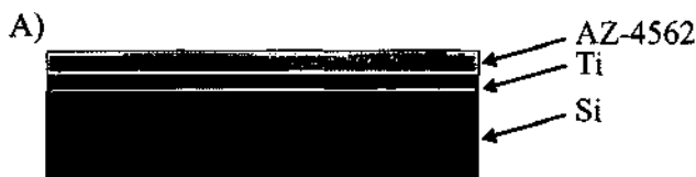
Fig. 3.10: Coating of the 40 \mu\text{m} thick resist layer onto the Ti coated Si wafer.
