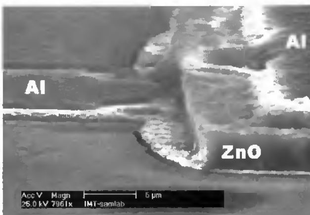
Fig. 2.19: Close-up view of the missing Al step on the ZnO layer.
