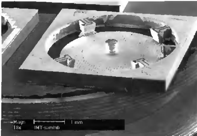
Fig. 2.17: Backside view of the microfabricated silicon stator with the anchor in the middle of the membrane and the T structures used to support the membrane during the two DRIE steps.
