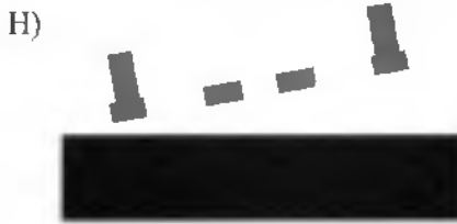
Fig. 3.31: Structures released by sacrificial etch of the Ti layer in HF.
