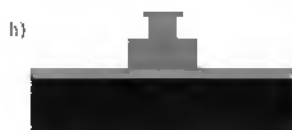
Fig. 5.17: Stripping of both resist layers.
