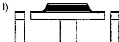
Fig. 2.13: Backside DRIE to liberate the membrane.
