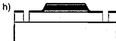
Fig. 2.12: Topside DRIE to define the silicon membrane.
