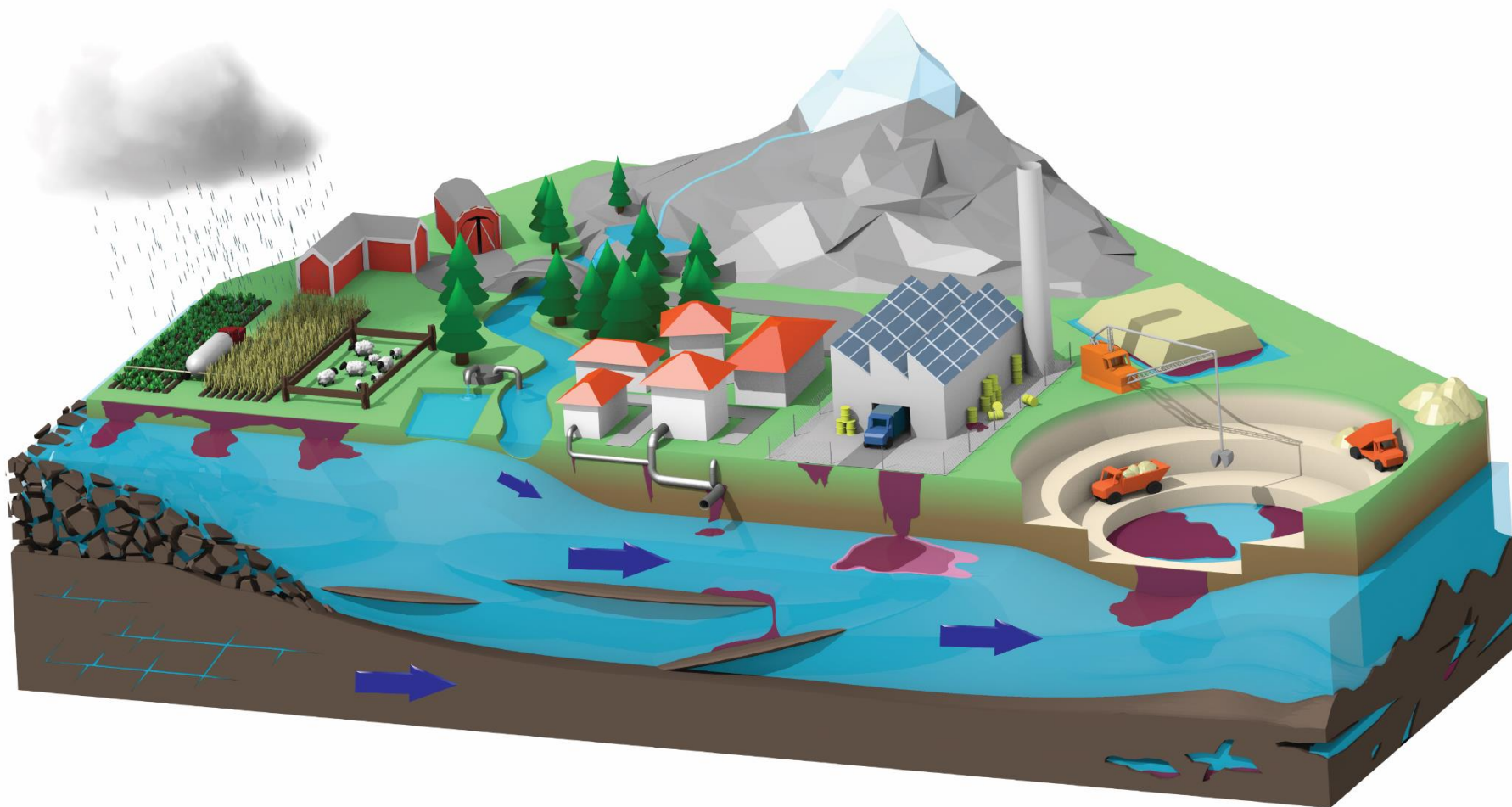
Figure 2-1. Sources of potential groundwater contaminants, as diffuse and point source inputs, from agricultural, urban and industrial settings and with respect to the dominant flow direction (arrows).
