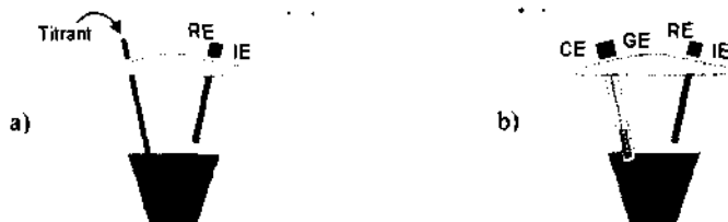
Fig 1.1. a) Volumetric batch titration, RE and IE stand for reference and indicator electrodes, respectively. b) coulometric batch titration, CE and GE are the counter and the generator electrodes, respectively.
