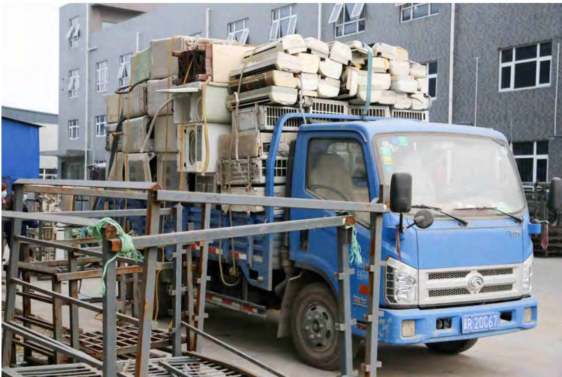
Figure 5.11: A truck delivers washing machines and air conditioners to a licensed DEEE recycling plant in Beijing. Appliances sold to licensed plants cannot be compressed because of subsidy requirements. Photo credit: the author.
