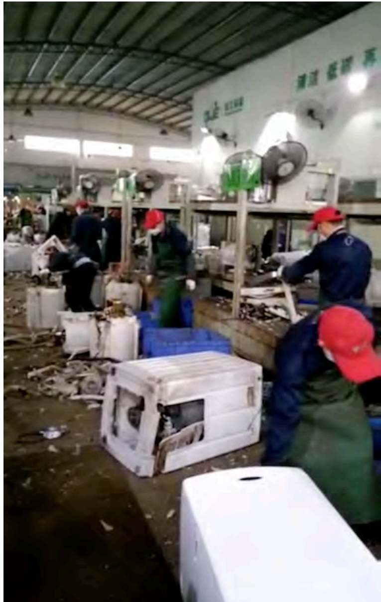
Figure 5.17: Still from a video shot by a factory worker in a licensed recycling plant in Qingyuan. Washing machines are dismantled manually, which requires grueling labor from the workers and exposes them to a high risk of injury. Photo credit: Mr. Chen.
