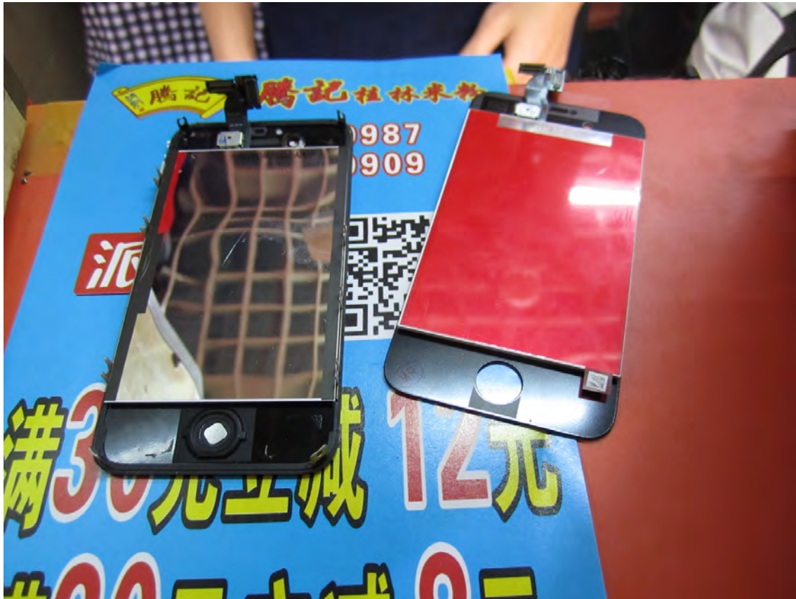
Figure 7.14: Left: an “original” ( yuanzhuang 原装) screen module for the iPhone 4. Right: a “high-quality replica” ( gaofang 高仿). Unlike experts, laypeople can find it very difficult to distinguish between the former and the latter. The workshop owner described the former as more “durable” ( naiyong 耐用) than the latter. Photo credit: the author.
