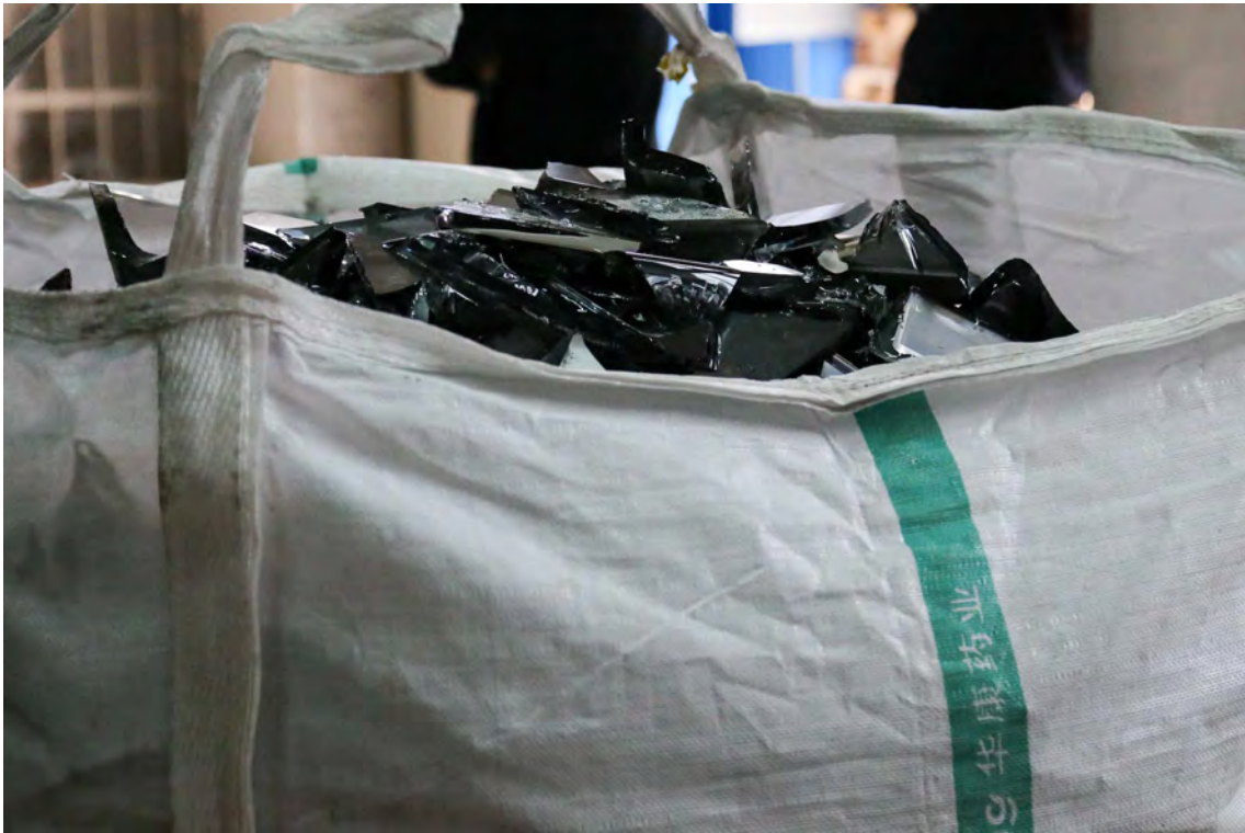
Figure 5.13: Broken CRT glass in an industrial “big bag”. As a rule, licensed DEEE recycling plants do not process this fraction on site. Photo credit: the author.
