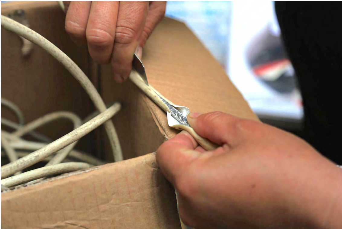
Figure 6.12: A junk collector in downtown Guangzhou cuts an electrical cable open in order to remove the copper wire from the plastic and iron sheaths. Photo credit: the author.
