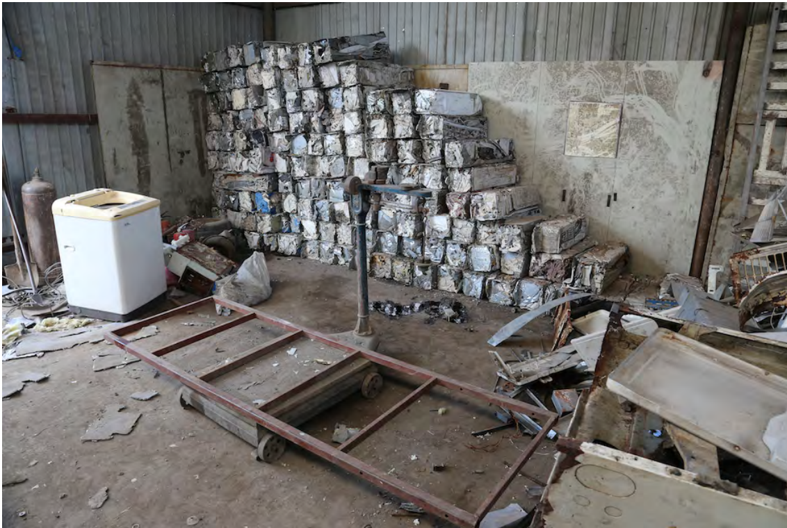
Figure 5.10: In this workshop located in the outskirts of Beijing, washing machines are dismantled and metal parts are compressed. That way, they take up less space and trucks can carry more scrap to processors. Photo credit: the author.
