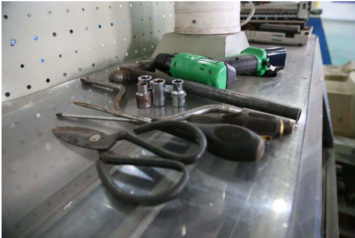
Figure 5.18: The type of tools with which a considerable part of the incoming DEEE is dismantled in licensed recycling plants. Photo credit: the author.
