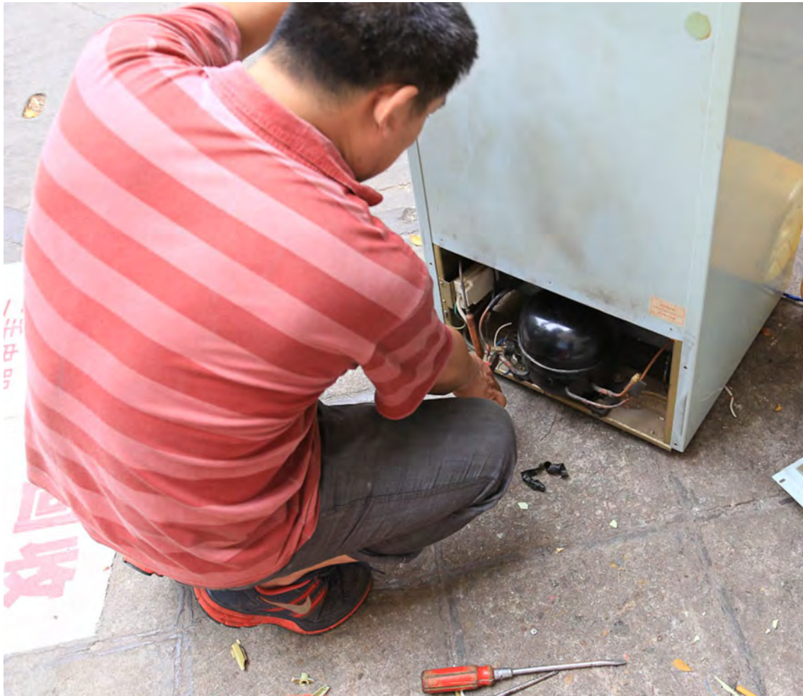
Figure 6.9: A junk collector in downtown Guangzhou removes a compressor from an old refrigerator. Photo credit: the author.
