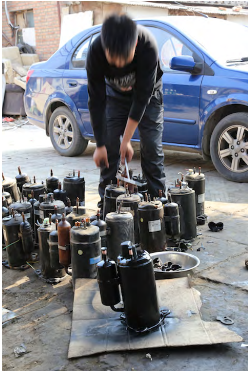
Figure 7.3: A young man refurbishes compressors from air conditioners in the outskirts of Beijing. Photo credit: the author.
