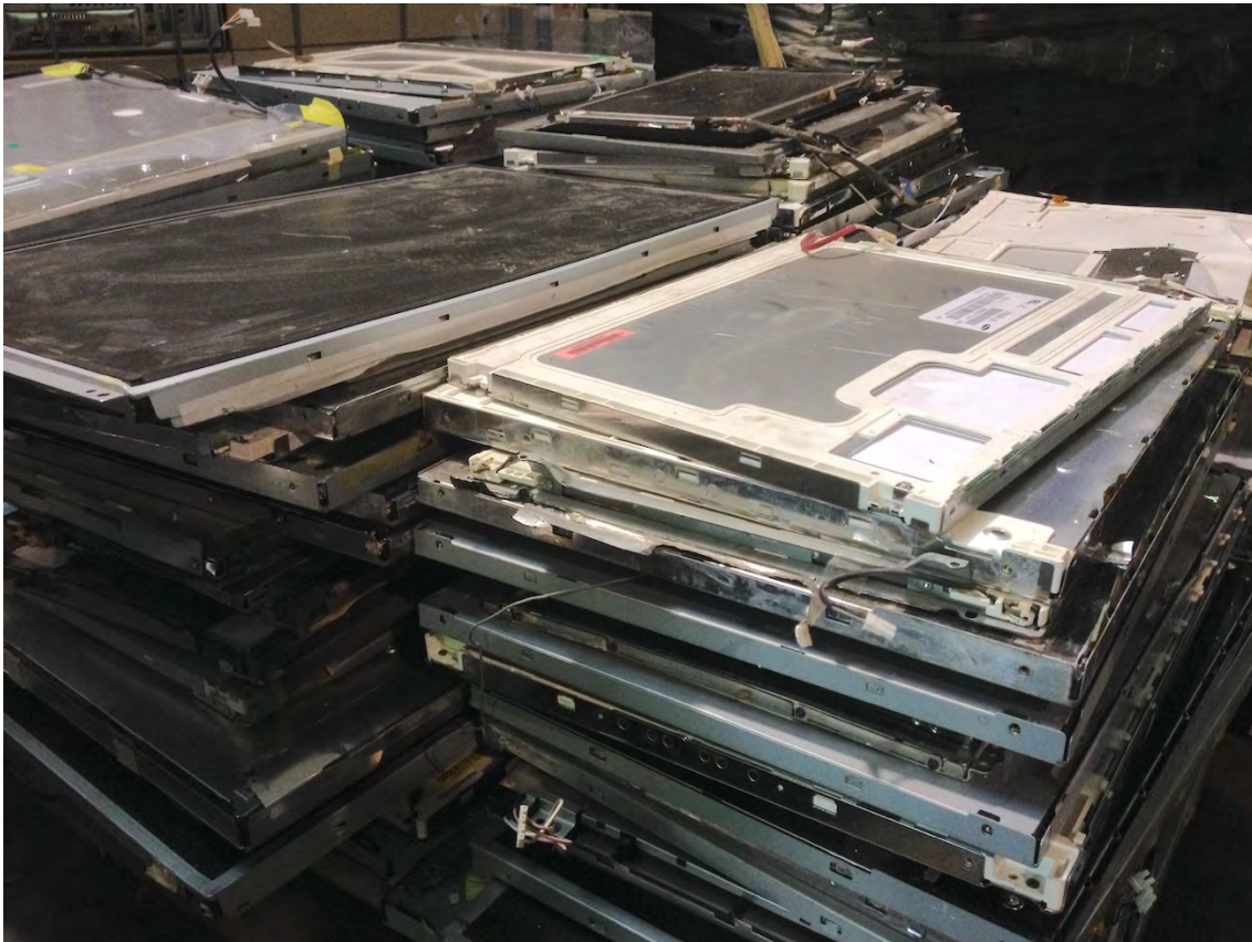
Figure 7.20: FPDs piled up after they have been extracted from monitors in an Italian recycling plant. Photo credit: the author.
