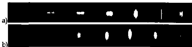
Fig. 5.14: Images of the focused beam at different positions along the optical axis. Focused with a microscope objective (a) and an anamorphic diffractive lens (b).
