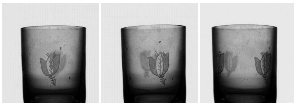
Fig. 5.20: SWIR images at 1906 nm for V model cup aged for 17 months in three different orientations (Field of view: 9 cm \times 8 cm)
