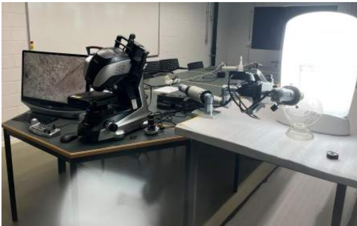
Fig. 5.3: Keyence digital microscopy setup along with flexible arm being used for imaging the neck region of LM15473 in transmitted light (©SNM)
