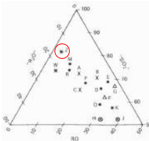
Fig. 3.1: Ternary state diagram with processed glass analyses of different glasses. Stable glasses (A, M, R) lie approximately in the middle of the diagram, glasses that are very susceptible to corrosion (H, J, Q) are at the lower right edge. W and Z show damage even in the museum. The remaining glasses show various corrosion phenomena [1]
