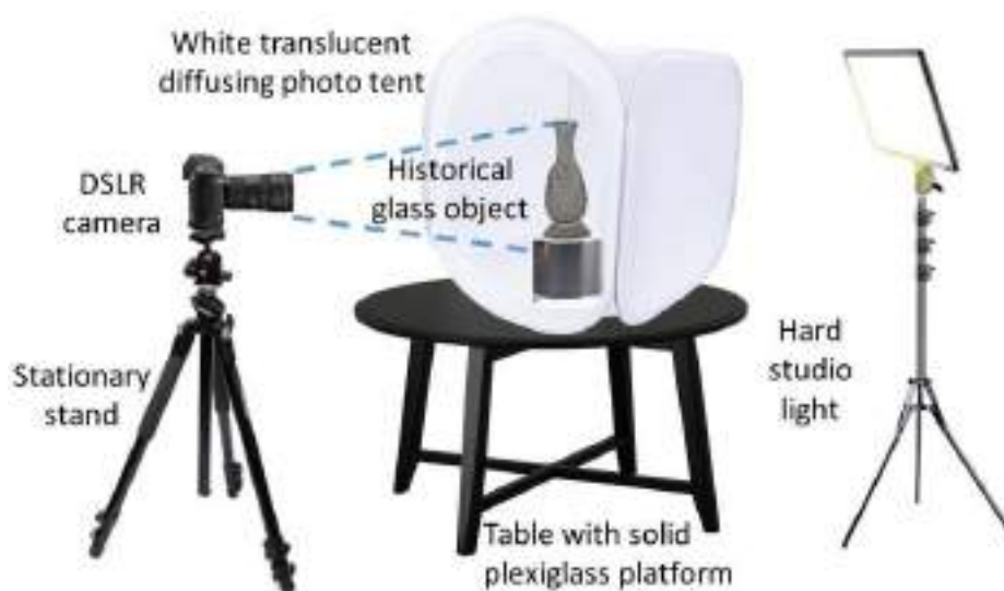
Fig. 5.1: Schematic diagram of the photography setup for the 3D glass objects
