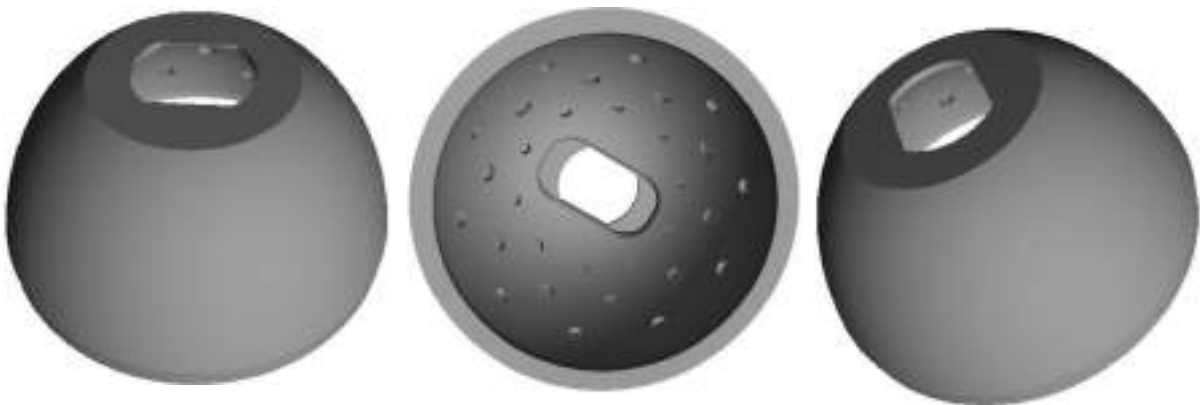
Fig. 2.25: Black plastic background designed for RTI acquisitions of model glass.
