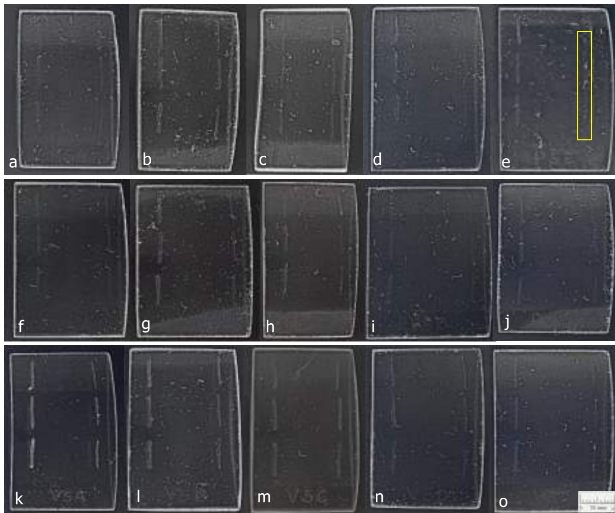
Fig 3.9: TCPL images of P model glass aged for a) 3 b) 6 c) 9 d) 12 and e) 17 months, PV model glass aged for f) 3 g) 6 h) 9 i) 12 and j) 17 months and V model glass aged for k) 3 l) 6 m) 9 n) 12 and o) 17 months
