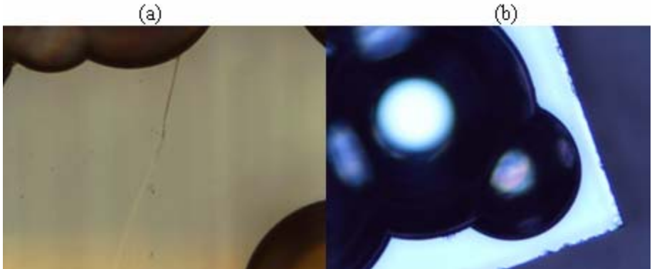
Figure 4.7 Top view of glass lid of failed samples inspected under an optical microscope (scale approximately 500\mu\text{m} ). (a) visible crack in the top of the glass lid. (b) pit in the top of the glass lid, due to a hole in the etch mask. The pit clearly does not penetrate all the way through the glass. Similar defects could be observed on passed samples. These observations do not explain the failures.
