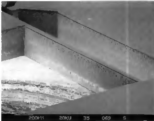
Figure 4.15: SEM picture of a suspension beam: 2000\ \mu\text{m} long, 40\ \mu\text{m} wide and 377\ \mu\text{m} thick.
