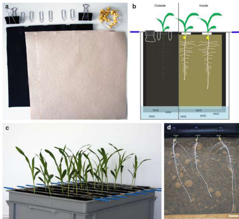
Figure 1. Fig. 1 Details of the SF-ROBS. (a) Elements of the pouch system with germinated maize seeds in the upper right corner. The SF-ROBS consists in pouches formed from black PE foil folded on itself and two humid filter papers. The layers are held together by paper clips. These pouches are attached to an aluminium rod with two foldback clips and placed in polypropylene containers that contain the maize nutrient solution (MNS). (b) View of the outside and the inside of the black PE foil pouch in which plants are growing. (c) Nine-day old maize plants. (d) Root systems of 5-day old plants in the SF-ROBS. Bar = 2 cm.
