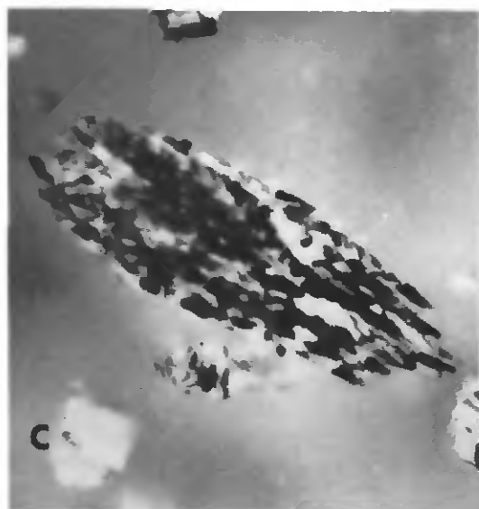
Fig. 7. Sequence of nucleation of the lamellar eutectic colony; annealing at 260°C: (a) isolated needle of orthorhombic boride; (b) single crystal nickel forms on the boride needle; (c) multiple-lamellar eutectic colony.
