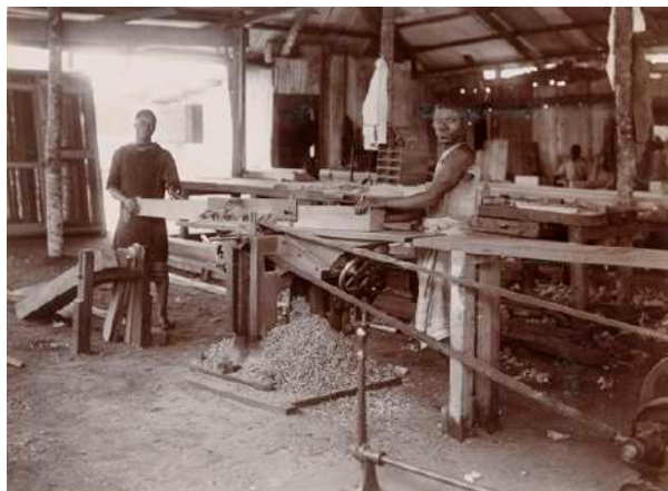
Fig. 10.75 RCSPC-Fisher Workshop, Planing and moulding machine . Public Work Department. Uganda, 1917
