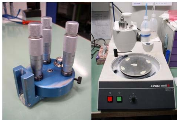
Figure 2.13: Left: Tripod used for wedge etching sample preparation / Right: rotative plate Struers LaboPol-4.
