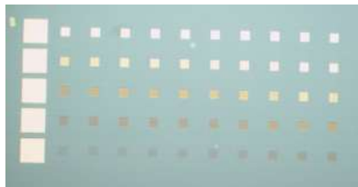
Figure B.13: Optical microscope image, Si substrate, 10s prebake, exposure dose 60\mu\text{C}/\text{cm}^2 . Green-gray background is unexposed resist. Big squares on left side are 50\mu\text{m} \times 50\mu\text{m} and fully cleared, i.e. the resist is entirely removed. Small squares changing color from dark brown, over yellow to bright brown indicate the evolution from insufficient dose which only exposes partially the resist layer to sufficient dose which entirely removes the resist.
