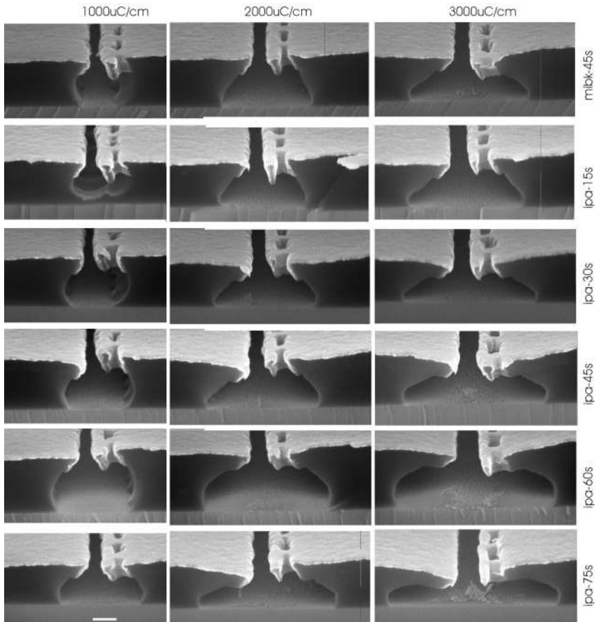
Figure 5.32: Undercut profile function of dose and developer. SPL dose 1000 through 3000 \mu\text{C}/\text{cm} , top MIBK+IPA=1+3, others IPA+H 2 O=9+1. The lower right side SEM pictures show a cave in effect of the resist bridges. This is not a mechanical issue, it is due to the interaction of the scanning electron beam acquiring the picture with the sample, and cumulative, i.e. getting the worse the more images are captured. Scalebar=100nm.
