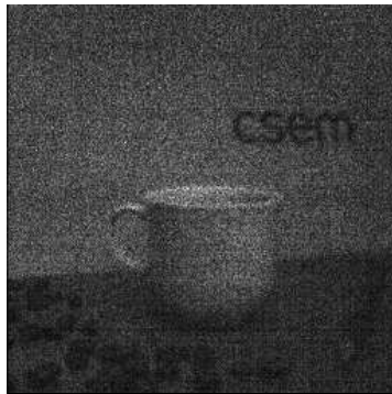
FIGURE 3.25 Row temporal noise corrected and column fixed pattern noise corrected image with a maximum of 24 and an average of 6 photoelectrons per pixel
