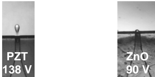
Figure 2.8: Stroboscopic image of droplet and meniscus position at driving voltage given in table 2.4. ZnO was not able to push the droplet completely out of the nozzle because the pressure becomes important at that moment. Successful dispensing is achieved with PZT ceramic actuators.
