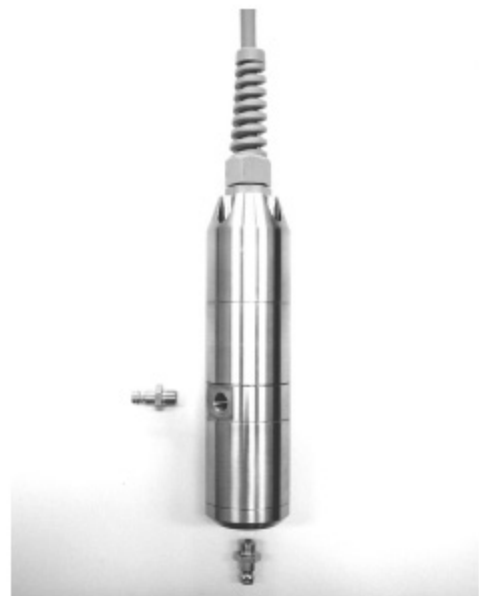
Figure 1. Two-inch diameter stainless steel fluorometer sonde with optional quick-connect fittings.
