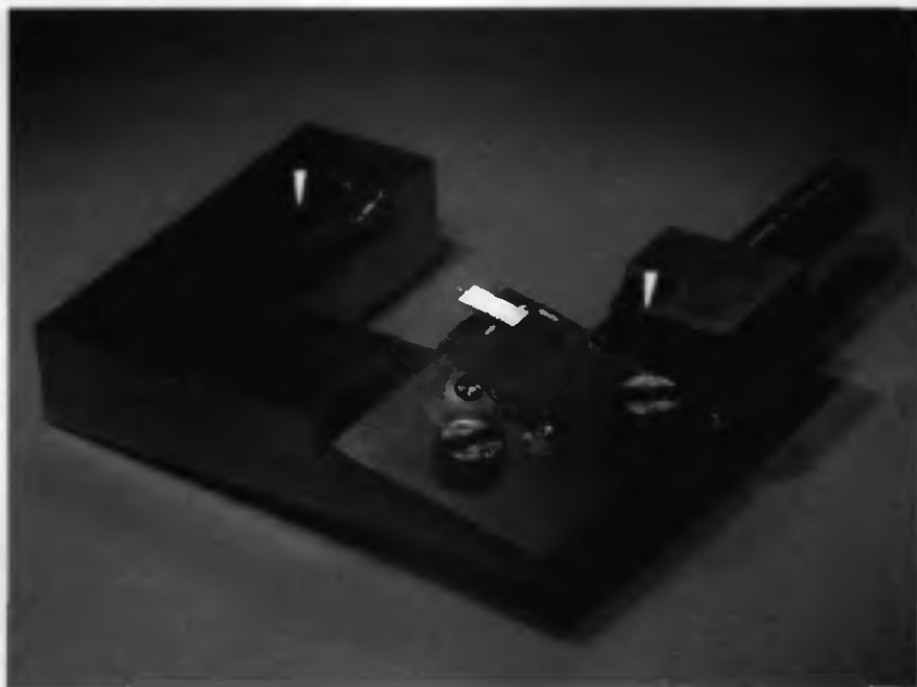
Fig. 6.4.1 Silicon chip with a 1000 \mu\text{m} long cantilever glued on a PCB with 5 metal lanes and screwed on a metal support. The ensemble can be fitted in a Nanoscope® III AFM head.
