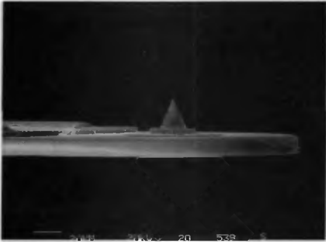
Fig.6.2.8. Released cantilever with sharp tip and side-by-side zinc oxide lanes for lateral force detection.
