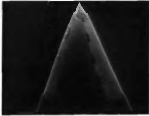
Fig. 6.2.5 Partial nitride RIE etching. Silicon is protected by the thin underlying oxide layer. Note tip and edges effects. Scale bar is 2\ \mu\text{m} .
