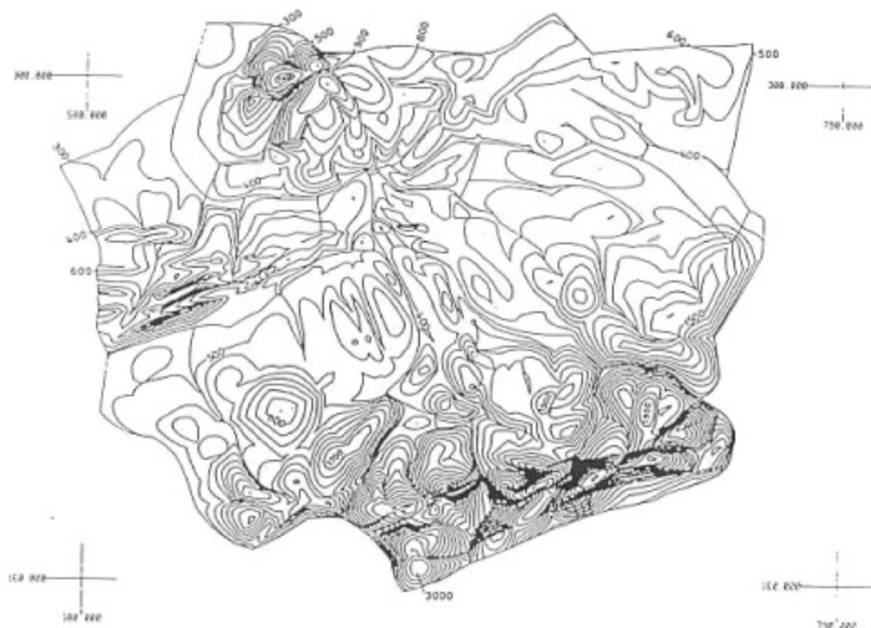
Figure 8. Example of fixed head boundary conditions imposed on the upper surface of the regional model.
