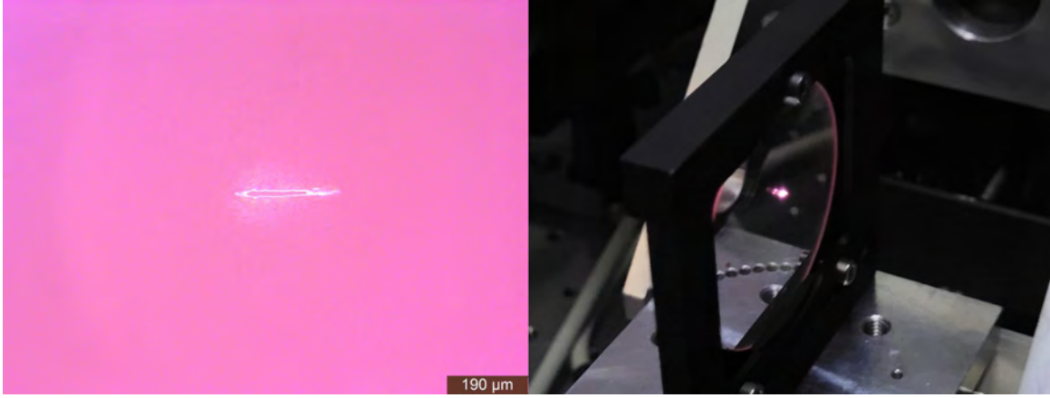
Figure 54: On the right side, you can see the damage induced in the substrate by the Kerr effect caused by the laser pulse from the LIDT measurement. On the left side, an overlay of 180 photos taken through the microscope with different depth focus points, which together show the filament induced by the Kerr-effect in the 2 mm thick substrate.
