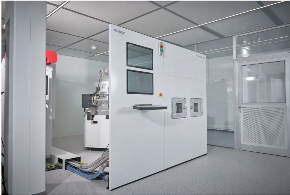
Figure 29: The front side of the used BPM Clusterline 200 is shown. On the left side is the control panel with the two screens and on the right side the two load locks. On the left behind the front, the rack with its service control panel can be seen behind the pillar.
