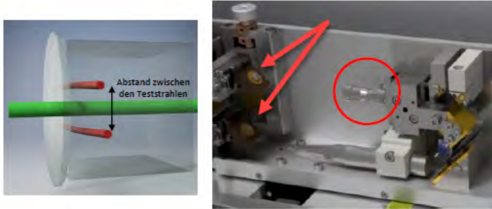
Figure 23: The figure shows on the left side the setup of beam path through the sample. On the right side the red arrows point on the sensors which measure the offset of the beam paths. The red circle shows where to calibrate the distance of the laser beams to the pump beam. The sample holder in the middle is removed. Figure adapted from the tools manual [21]
