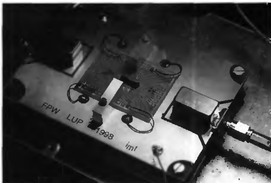
Figure 7.5: Optical view of the experimental setup. This configuration with two PCB levels, allow for stable device handling and minimal noise. An e.m. shield is placed between the contact lines of each balun, to suppress their direct capacitive coupling.
