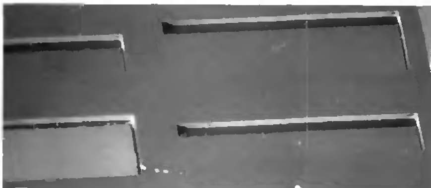
Figure 6.19: Photograph of four multilayer membranes (silicon nitride and platinum). Overall dimensions are 1 or 2 mm by 8 mm, while the thickness is 0.76 \mu\text{m} .
