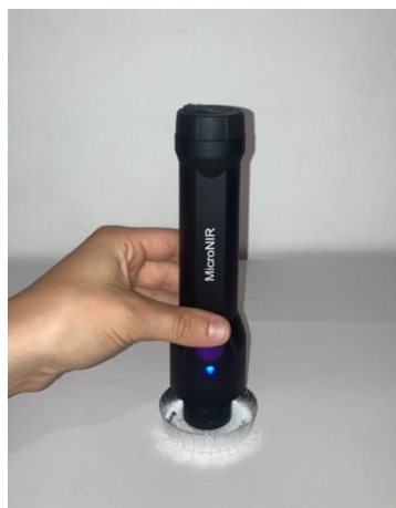
Figure 1. The microNIR device used to analyse all samples on a typical aluminium plate. In this specific example, the sample is crystalized sugar.
