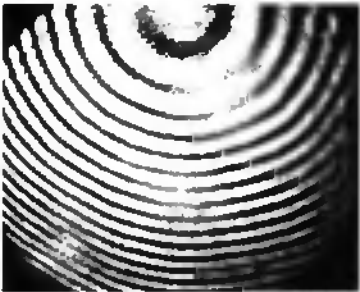
Figure 6.5: Interferogrammes around the targeted 2,2 mode at 212.5 kHz. The numbers correspond to the actuation frequency in kHz.
