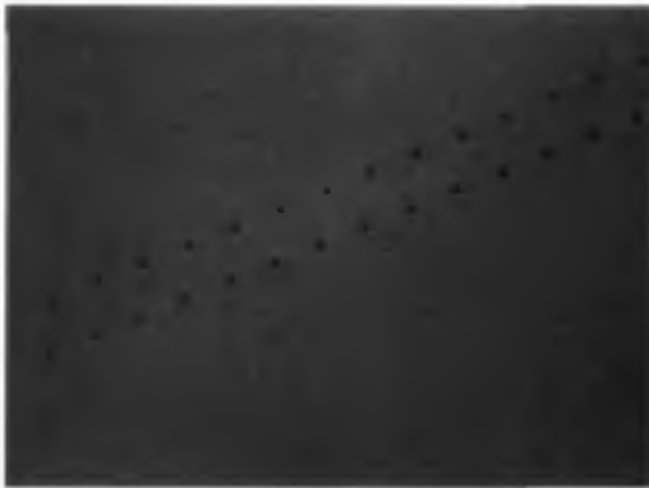
Figure 6.7: Overview of the nozzles in a Vapo8, nozzles were measured to be 8 \mu\text{m} in diameter.
