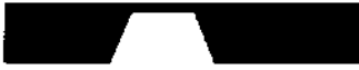
Thin membrane with 1) Nozzle etched with KOH from the front side. 2) DRIE etched nozzle
