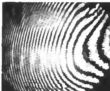
Figure 4.9: Interferogrammes of a device vibrating at 115.6kHz, taken with different amplitudes. The image is taken over the full front surface ( 10 \times 10 \text{ mm}^2 )
