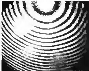
Figure 6.5: Interferogrammes around the targeted 2,2 mode at 212.5 kHz. The numbers correspond to the actuation frequency in kHz.
