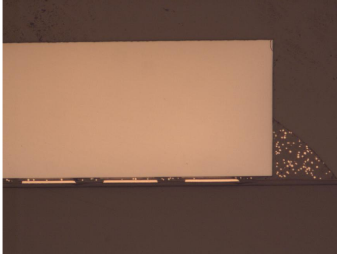
Figure 4.12: Cross section of a flip chip ACA-joint on a PMMA substrate. The bonding force is 400 g and the bonding temperature of the chip 90 °C. No deformation is visible.
