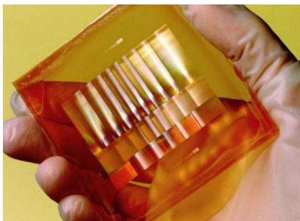
Fig. 1. Lenslet array recorded in photoresist for custom IR detector application.
