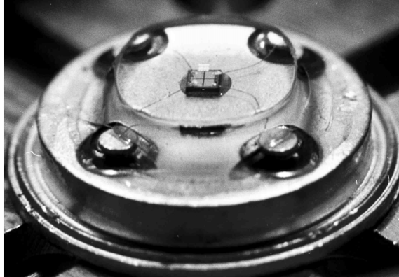
Figure 5.10: 2x2 VCSEL array mounted on a TO-39 package header with diffractive lenses, replicated in ORMOCER for multimode fiber coupling.
