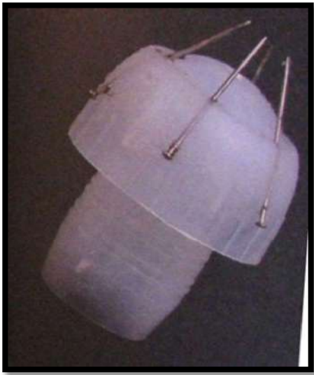
Figure 8. Berry-piercer for making jam, made out of a champagne plastic cork and needles. Author: Nikita Kuzmichyov. Moscow. 1987. Reproduced in: Arkhipov 2003, 66
