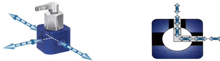
Figure 6.1 Hamilton AG three-way actual mechanical microvalve measuring about 10 cm 3 .
