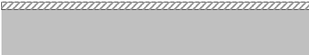
Figure 8.16 A 5000 \text{\AA} thermal \text{SiO}_2 mask is grown on both sides, to be removed from the backside in a subsequent step.
