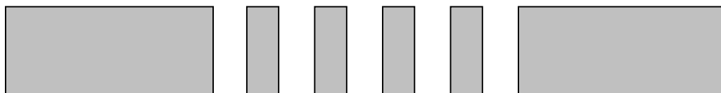
Figure 8.3 Plasma O 2 photoresist removing, and etching of aluminum to free the structures.
