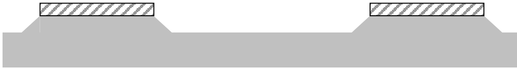
Figure 8.14 A KOH solution thins the wafer from 525 \mu\text{m} to thicknesses within the range of 410 to 450 \mu\text{m} .
