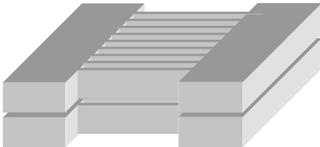
Figure 7.2 Schematic close-up view of the beam structure. Hundred of high-aspect-ratio beams are arranged in parallel.
