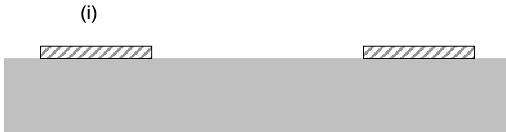
Figure 8.13 A 5000 Å thermal SiO 2 mask is patterned on the topside.
