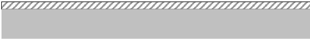
Figure 8.17 The silicon wafer is thinned down to 420 \mu\text{m} .
