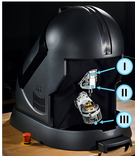
Fig. 2 Micro 5 machine with accelerometers & acoustic sensors locations. (Reprinted with permission, courtesy of Guillaume Perret; This figure is not included under the article's CC BY license.)
