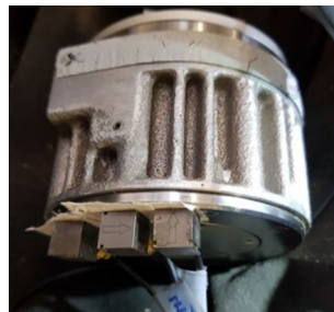
Fig. 2 Micro 5 machine with accelerometers & acoustic sensors locations. (Reprinted with permission, courtesy of Guillaume Perret; This figure is not included under the article's CC BY license.)
