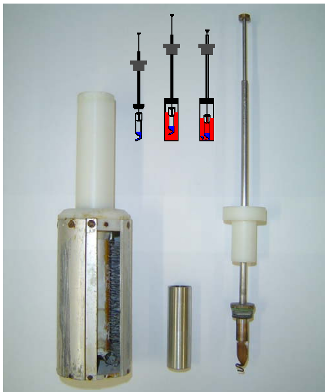
Figure 7. Immersion calorimeter: main part with the 180 thermocouples (left), the tube containing the liquid (centre) and the sample holder with the outgassed sample (right). The inset shows the filling of the sample holder following the breaking of the capillary at the bottom. The enthalpy of immersion is monitored by the voltage difference in the thermocouples V(t) .
