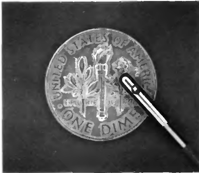
Fig. 6.1 Piezoresistive pressure sensor mounted in a 6F heart catheter.
