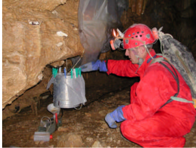
Figure 21: the pluviometer installed at EC is used for discharge measurement. At the outflow a conductivity-temperature probe is connected to a datalogger.
