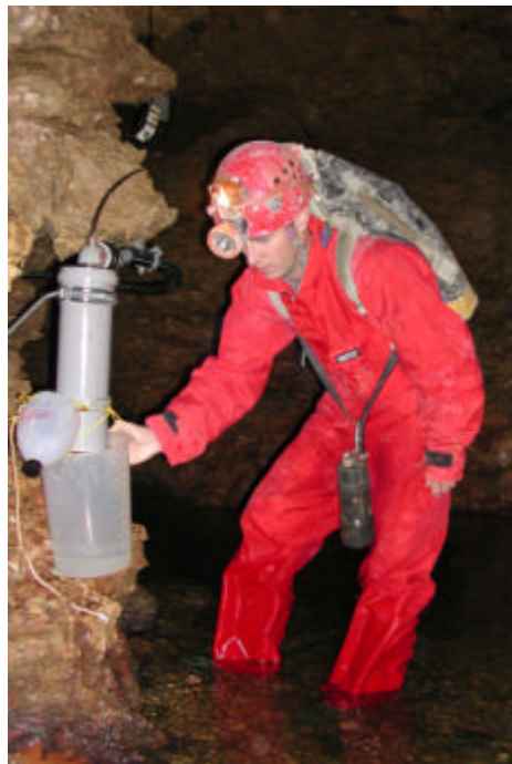
Figure 22: SO tributary is collected into a pipe. At its end, discharge is continuously measured by a super pluviometer (grey PVC tube on the picture).
