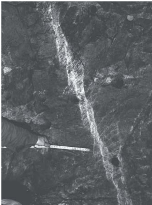
Fig. 2. Shear rupture consisting of an echelon array of tensile microcracks produced at higher confining stress levels [15]. This is analogous to shear planes formed in triaxial compression tests.
