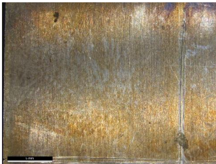
Figure 4.30 Optical microscope observation of silver sample after application of an EDDS-agar gel and rinsing with a cotton swab. Scale bar indicates 5 mm.
