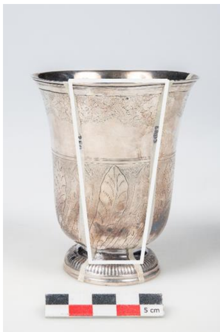
Figure 4.32 Silver cup lent by the Musée Dobrée after treatment, centered on the EDDS-treated part (white trapezoid).
