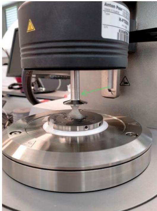
Figure S3.3 Set-up for the tack test measurements on xanthan gum, probe increasing and stretching the material, showing a cohesive rupture.
