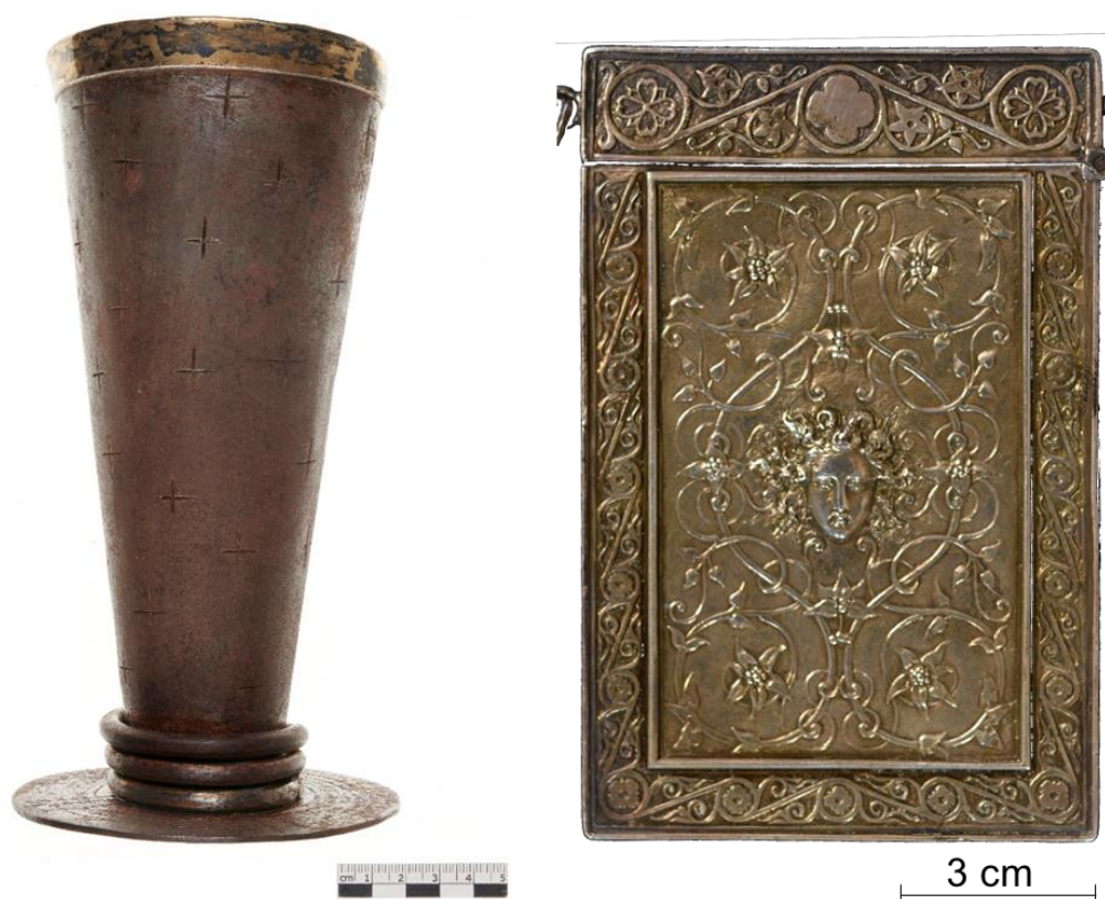
Figure 3.18 Calix (left) and card-holder (right) used as sacrificial objects for the detection of gel residues amended with fluorescent markers.
