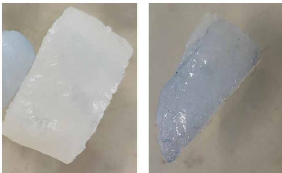
Figure 4.16 CS-ItA-LCys gels after before (left) and after (right) application on NAC samples.
