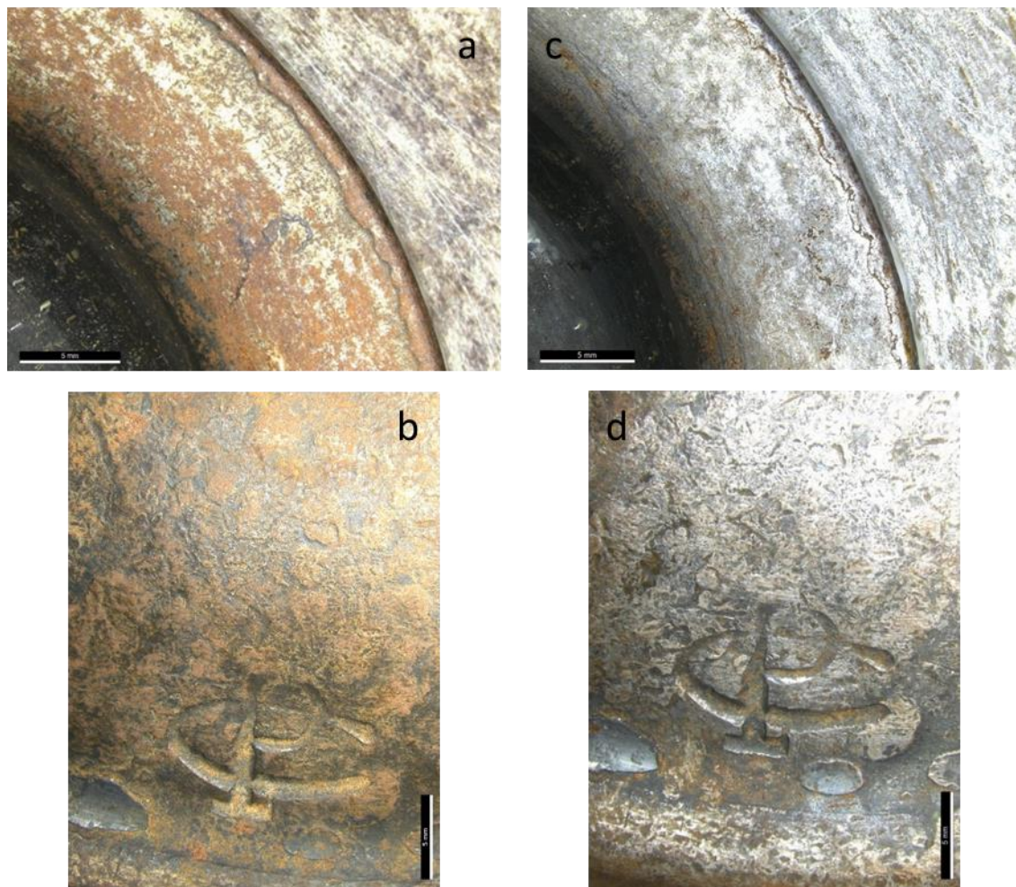
Figure 4.8 Digital microscope images of details from the candleholder before (a, b) and after (c, d) cleaning with 6 \cdot 10^{-2} M DFO-amended agar gels. Scale bar indicates 5 mm.
