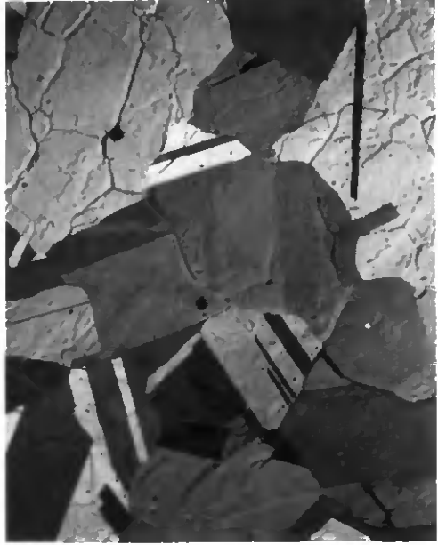
Fig. 4d. 42 min d = 45 \mu\text{m}
