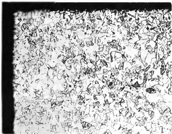
9 Corner of a sample annealed at 750°C for 2 h in an air furnace, as viewed in the OM. No grain coarsening has taken place. \times 50 .
