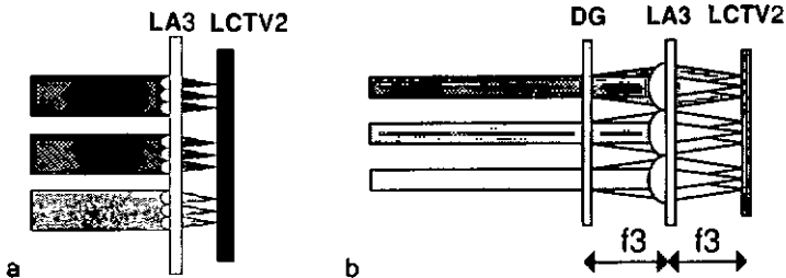
Fig. 2.21: The replication of each individual channel (interleced fan-out) can be made using the same concepts as for the other fan-outs that have been discussed so far. Advantages and problems apply respectively.
