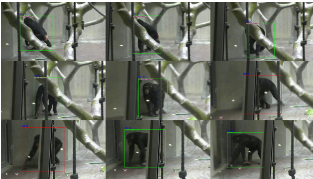
Figure 2. Tracking example after interpolation for missing frames (red bounding box) and corrected ID. As the individual passes behind the pole, its track was lost and the ID was swapped with another.
