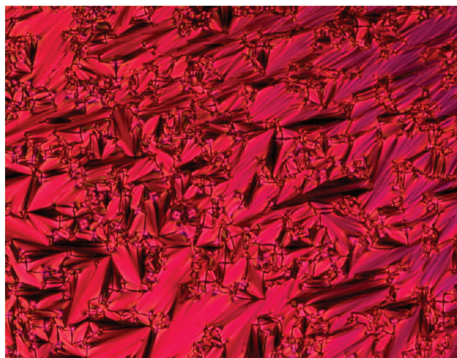
Figure 2. Thermal optical micrograph of the focal-conic fan texture displayed by BOD-G 3 in the smectic A phase at 161 °C.
