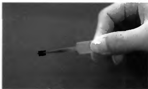
Fig. 1.2: Chip with silicon cantilever and tip held by tweezers. The picture demonstrates how a series of transducers are used to bridge the gap of 9 orders of magnitude between the human dimensions ( 10^0 m) to the nanometer scale world ( 10^{-9} m).
